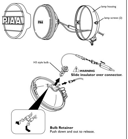
When service is complete reverse steps to assemble lamp. Make sure to not pinch wire while assembling.
